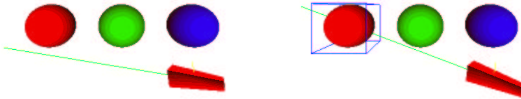
Figure 2.3: Selection of a virtual object with ray-casting, where the ray emanating from a manipulator like the wand does not intersect (left picture) and intersects (right picture) with a virtual object.
